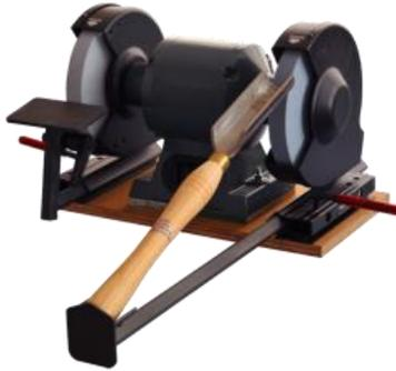
*Figure 11 Bench Grinder with Wolverine Sharpening System*
