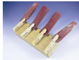
Clothespins epoxied to a board work great for holding strips of sandpaper. Write the grit number on each clothespin to keep the different grits separated and within easy reach.
