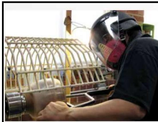
Turning with the wire guard in place, wearing my riot helmet and respirator. The piece, which has multiple cracks, is wrapped in plastic stretch wrap for reinforcement.
