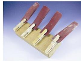
Clothespins epoxied to a board work great for holding strips of sandpaper. Write the grit number on each clothespin to keep the different grits separated and within easy reach.
